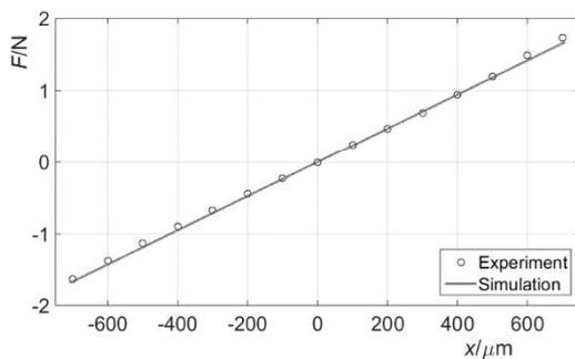
Figure 2.  $F$  vs.  $x$  characteristics of the actuator.
