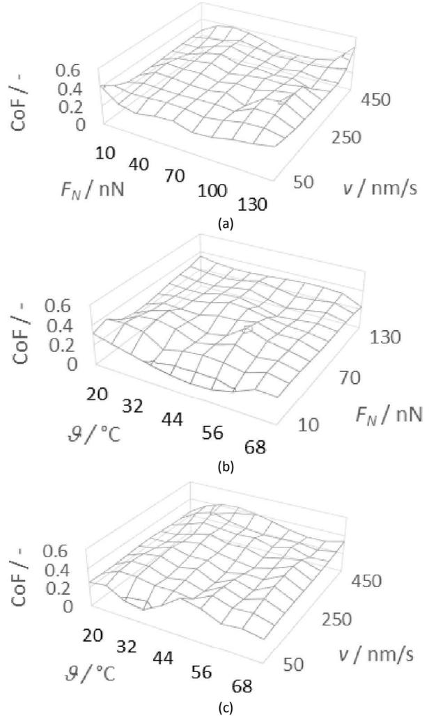
**Figure 1.** CoF values on a  $\text{TiO}_2$  sample with fixed:  $\vartheta = 20^\circ\text{C}$  (a),  $v = 250\text{ nm/s}$  (b) and  $F_N = 50\text{ nN}$  (c).
