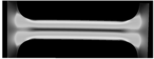
Fig. 6 FEM model of a streamline fillet
