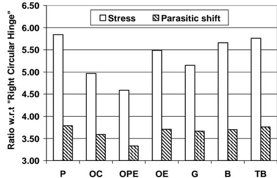
Fig. 7 Ratio of the normalized stress of the right circular (RC) hinge vs. that of the other hinges (white bars) and ratio of the parasitic shift of the various hinges vs. that of the RC hinge (hachured bars). P - prismatic beam hinge, OC - optimised circular hinge, OPE, OE - optimised elliptical hinges, G, B, TB – streamline hinges
