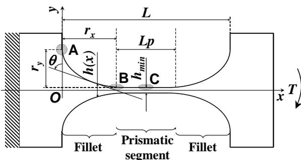
Fig. 5 General geometrical configuration of a flexural hinge
