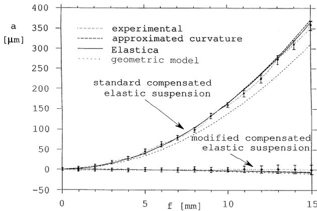
Fig. 4 Results obtained by using the proposed design methods to minimise the parasitic displacements of ultra-high precision positioning devices based on spring-strips
