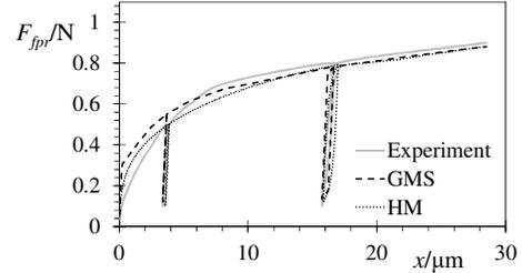
Figure 4. Comparison of experimental data with responses modelled via the GMS and HM friction models.
