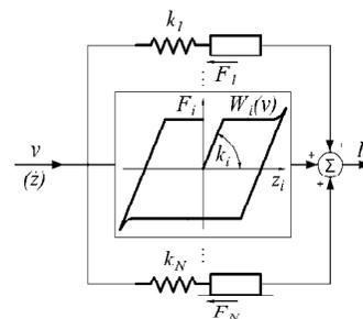
Figure 2. Schematic representation of the GMS slip blocks.
