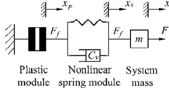
Figure 3. Schematic representation of Hsieh's friction model.
