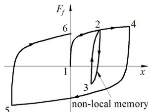
Figure 1. Pre-sliding friction behaviour.
