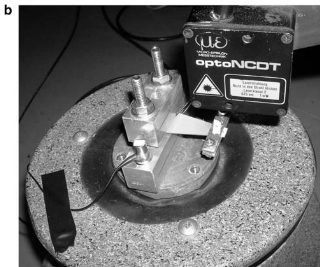
Fig. 12 Scheme of the experimental set-up (a): signal generator and amplifier (1), shaker (2), bimorph with proof mass (3), accelerometer (4), laser (5), resistive load (6); photo of the actual set-up (b)
