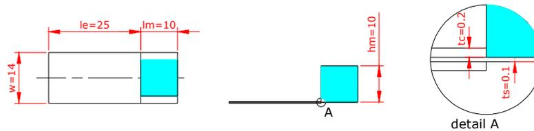
Figure 1: Reference rectangular piezoelectric energy scavenger.
