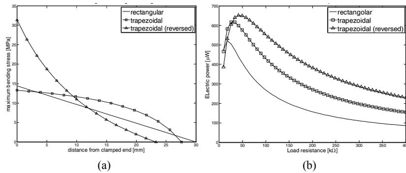
Figure 3: Comparison between the reference rectangular scavenger and optimised trapezoidal profiles with equal maximum widths. Maximum bending stress along beam length (a) and electric power generated via a resistive load (b).
