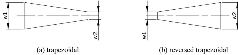
Figure 2: Optimised trapezoidal profiles with equal maximum widths.
