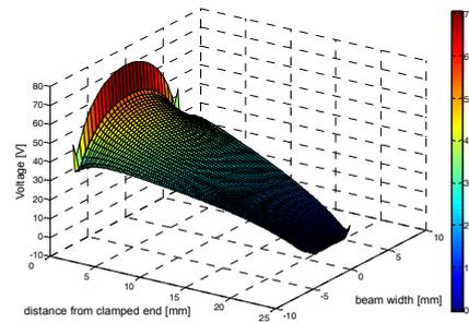
of the voltage obtained in the piezoelectric layers (Table 1) confirm the better performance of Design 1. In the case of the reversed trapezoidal layout of Design 2, the local stress concentration at the clamped end limits the possible increase of the average voltage value.
