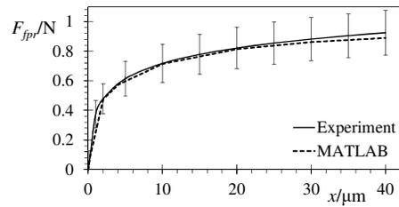
Figure 2. Experimental and modelled pre-sliding of the linear slide.
