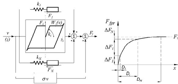
Figure 1. GMS model (left) and friction in pre-sliding (right).
