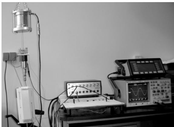
Fig. 8. Lay-out of the experimental set-up for dynamics measurements.
