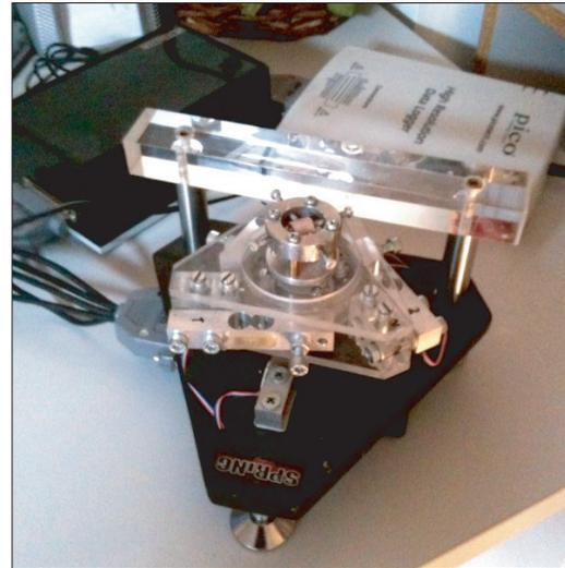
**Figure 4.** Torque-measuring device with mounted bone sample.
