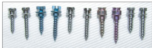
**Figure 2.** Tested mini-implants (from left to right): Dual Top™ (Jeil Medical Corp., Seoul, Korea) 1.4 × 6 mm, and 1.4 × 8 mm; Aarhus (MEDICON eG, Tuttlingen, Germany) 1.5 × 6 mm, and 1.5 × 8 mm; Dual Top™ 1.6 × 6 mm, and 1.6 × 8 mm; Ortho Easy® (FORESTADENT®, Pforzheim, Germany) 1.7 × 6 mm, and 1.7 × 8 mm; Dual Top™ 2.0 × 6 mm, and 2.0 × 8 mm.
