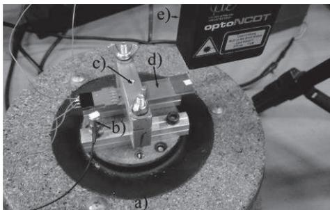
**Figure 3.** Experimental set-up: a) MB Dynamics shaker, b) Bruel&Kjaer 4375 accelerometer, c) cantilever clamping, d) Midé V21B scavenger, e) Micro-Epsilon Meßtechtechnik optoNCDT 1605 laser vibrometer
