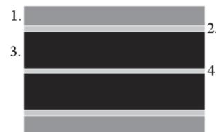
Figure 1. Layer structure of Midé Technology® scavengers: 1. FR4 layer, 2. Cu electrode, 3. piezoelectric layer, 4. ESPANEX layer
