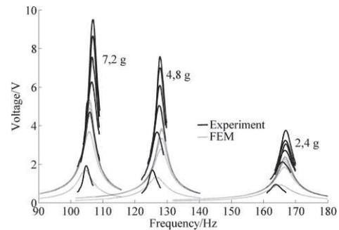
**Figure 4.** Comparison of experimental and numerical results for 12 electrical resistances and 3 tip masses for Midé scavengers type V21B
