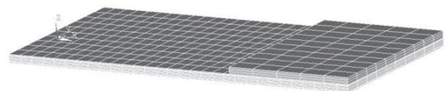
Figure 2. FEM structure of a Midé Technology® scavenger type V21B
