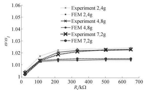
**Figure 5.** Comparison of numerical and experimental results of the electromechanical hardening effect for V21B Midé scavengers with three tip masses
