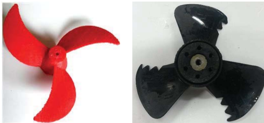
Figure 3. Propellers used in the experiments: narrow blades (left) and wide blades (right)
