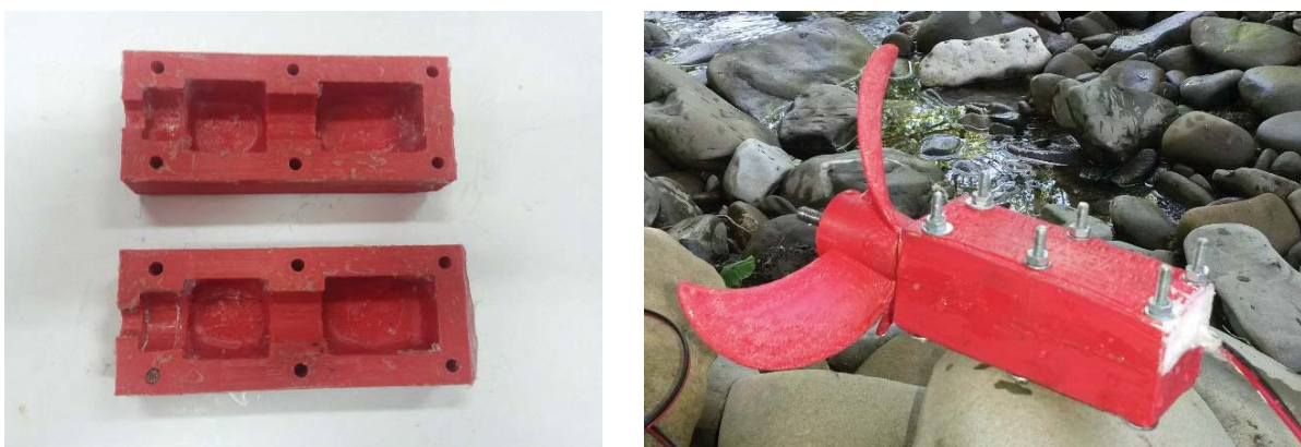
Figure 4. Printed parts of watertight enclosure (left) and assembly of miniaturised underwater hydro generator prototype (right)
