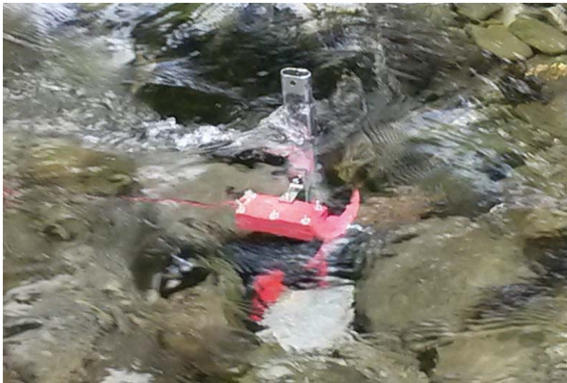
Figure 6. Miniaturised underwater hydro generator anchored in the Rječina river
