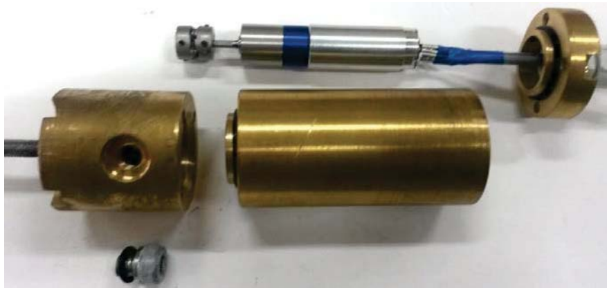
Figure 9. Final miniaturised underwater hydro generator
