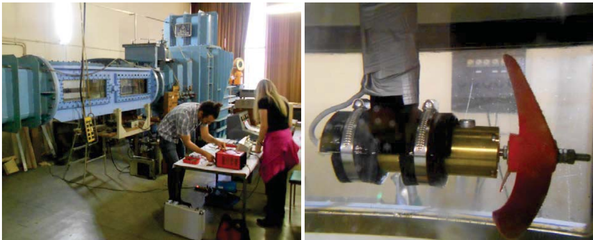
Figure 10. Flow tunnel assembly (left) and miniaturised underwater hydro generator in the flow tunnel (right) at the Naval research institute in Zagreb, Croatia
