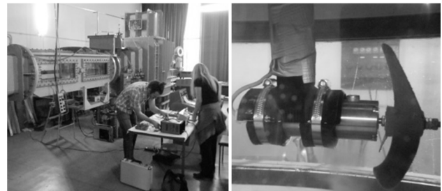
Figure 6. Flow tunnel (left) and hydro-generator in the flow tunnel (right)
