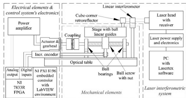
Figure 1. Simplified scheme of the considered positioning system.
