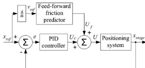
Figure 2. PID controller and additional feed-forward control block.
