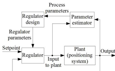
Figure 3. Scheme of the adaptive STR controller.
