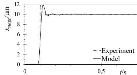
Figure 4. 10  $\mu\text{m}$  point-to-point positioning with STR adaptive control.
