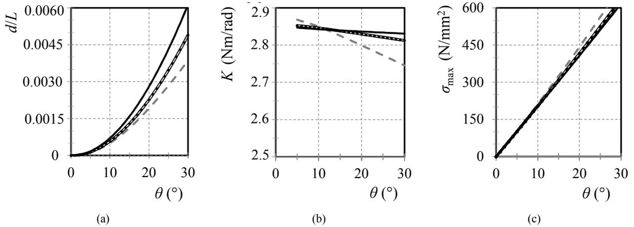
Figure 9. Change of  $d/L$  (a),  $K$  (b) and  $\sigma_{max}$  (c) versus rotation  $\theta$  for a monolithic pivots' configuration with  $\alpha = 15^\circ$  (dashed line),  $\alpha = 30^\circ$  (compound line) and  $\alpha = 45^\circ$  (solid line).
