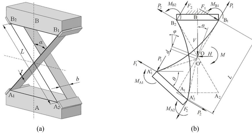
Figure 2. Characteristic dimensions of the cross-spring pivot (a) and schematics of the pivot in deformed position (b).
