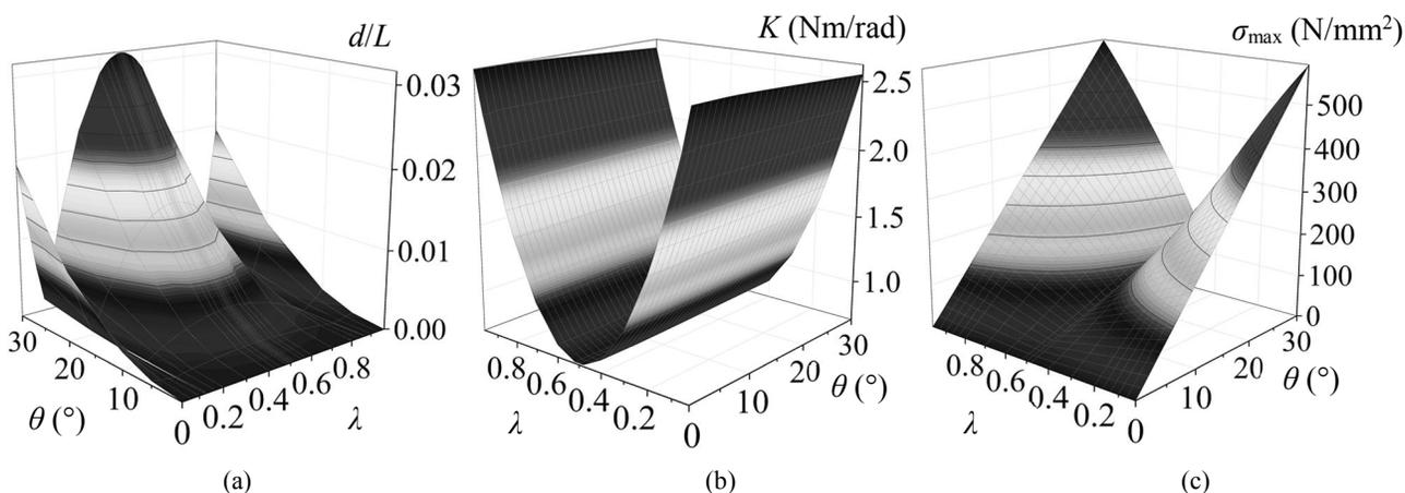
Figure 8. Change of normalised parasitic shift amplitudes (a), rotational stiffness (b) and stresses at spring-strips' fixed ends (c) versus rotation  $\theta$  depending on parameter  $\lambda$  for a design configuration with  $\alpha = 45^\circ$ .
