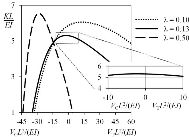
Figure 10. Rotational stiffness depending on vertical loads for various values of the geometric parameter  $\lambda$  when  $\alpha = 45^\circ$ .
