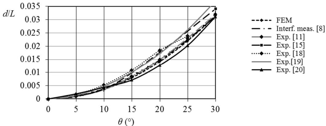
Figure 4. Comparison of normalized parasitic shift amplitudes  $d/L$  obtained via the FEA model with experimental results.
