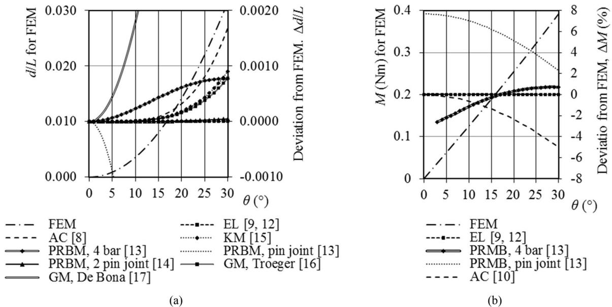
Figure 5. Comparison of FEM and results of various analytical methods in terms of normalised parasitic shift amplitudes (a) and couples (b) vs. rotation angle  $\theta$ .
