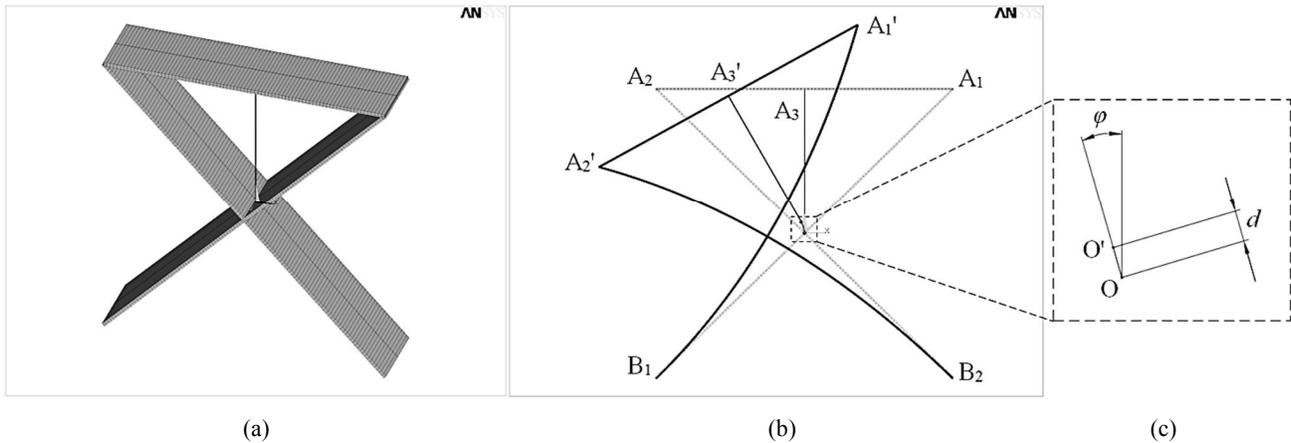
Figure 3. Meshed finite element model (a), deformed FEM of the cross-spring pivot (b) and its parasitic shift (c).
