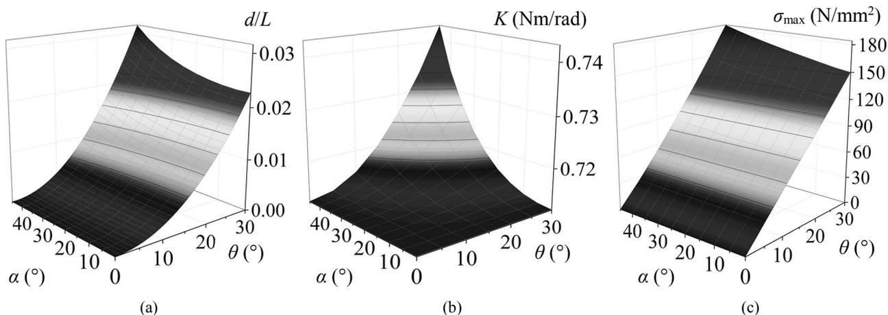
Figure 7. Change of normalised parasitic shift amplitudes (a), rotational stiffness (b) and stresses at spring-strips' fixed ends (c) versus rotation  $\theta$  depending on the inclination  $\alpha$  of the springs.
