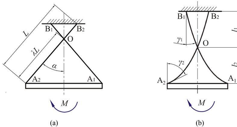
Figure 6. Variants of the cross-spring pivot design.
