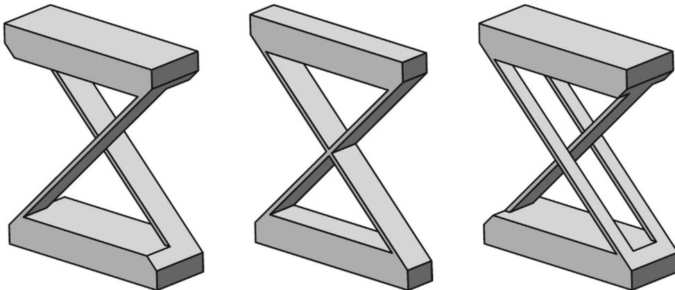
Figure 1. Different design configurations of a symmetrical cross-spring pivot.
