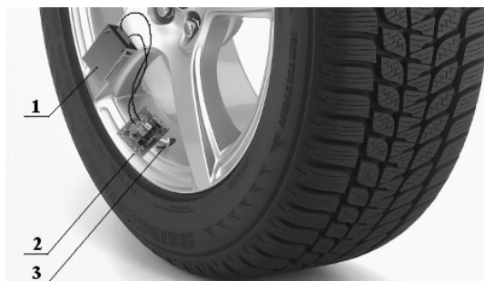
Figure 2: WTPMS concept: 1) piezoelectric scavenger with conditioning electronics, 2) TPM, 3) standard Schrader valve
